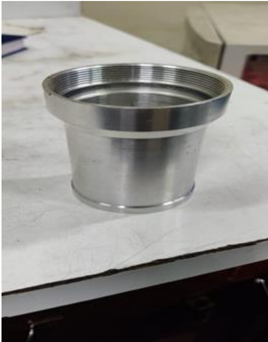
Fig: 20. Bush component after manufacturing at CNC machine-1
