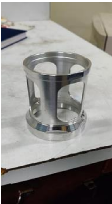
Fig: 22. Bush Component after manufacturing at CNC machine-2
