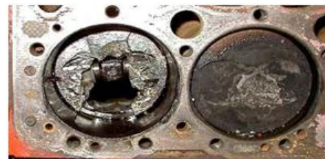
Fig 5.1.1 Damage from a piston striking a valve
